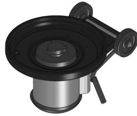
3. Use the four screws in the bag and mount the brush cover. Hand-tighten the screws first and then use a wrench to tighten them firmly. Use a CROSS pattern to tighten the bolts as shown below.
