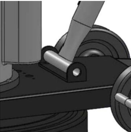
8. Insert the pivot axle screw (C22558) through the handle bracket and the handle pivot tube. Hand tighten the nut (C13100) to the pivot axle screw and finish by tightening with a wrench.
