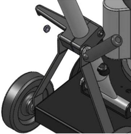
4. Put the locking clamp handle in the unlocked position (pointing up) and start tightening the nut C11558 on the threaded portion of the spade bolt (C11536).
