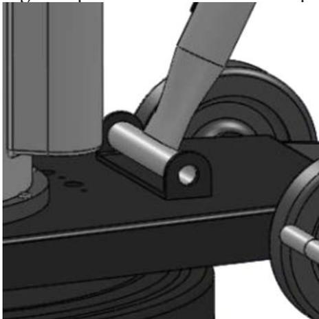
6. Place the handle in the down position to check the locking function. If too tight, unlock the handle and loosen the nut (C11558) slightly. If too loose, unlock the handle and tighten the nut (C11558), as needed. You have assembled the cord hook clamp assembly properly when the locking handle locks firmly in the DOWN position and unlocks and slides easily in the UP position.
