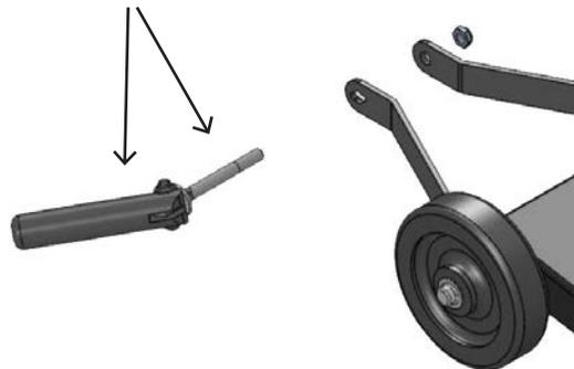
3. Insert the locking clamp handle/spade bolt assembly through the Cord Hook Clamp assembly (located on the handle) and the left and right handle braces ( D11481, D11482).
