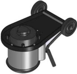
2. Pull out the brush cover from carton 3 and align the four holes on the brush cover to the four holes on the motor.
