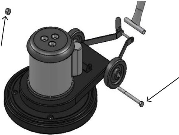
7. Insert the pivot tube at the lower end of the handle between the handle bracket on the base frame and align the holes to one another.
