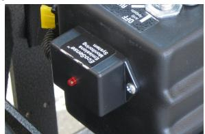
The monitor must receive a signal from the oxygen sensor in order to function. If it did not have a minimum reading requirement it would be possible to disconnect the oxygen sensor and operate the unit, even if the emissions were out of limits. In order for the unit to work as designed it must be able to read both low and high signals, with "not to exceed limits" of both.
