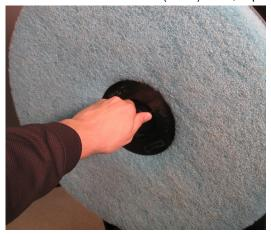
**CAUTION!** Carefully inspect the pad holder for cracks or damage. Replace if necessary.
