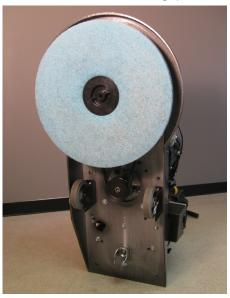
5. Remove centering device and inspect pad. If pad has worn to less than a 1/4" (6mm) thick, replace it.
