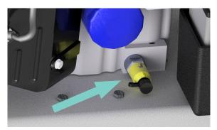
**Note:** In order for the oil to drain, it may be necessary to loosen the oil fill cap.
