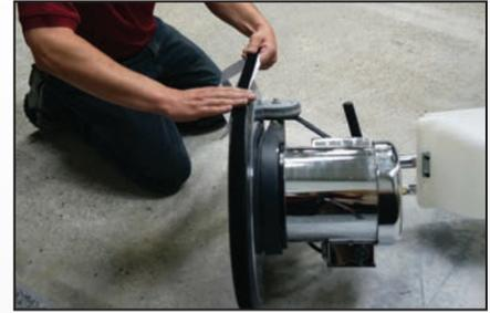
3. Apply VELCRO® strip to the middle/upper half of the outside diameter of the floor machine housing (bumper).
