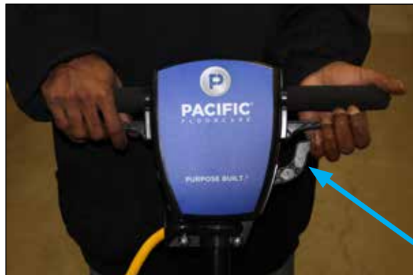
Adjusting handle height using handle adjustment lever
