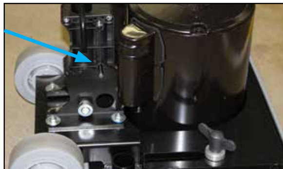
Handle locking mechanism in upright operation/ storage/transport position
